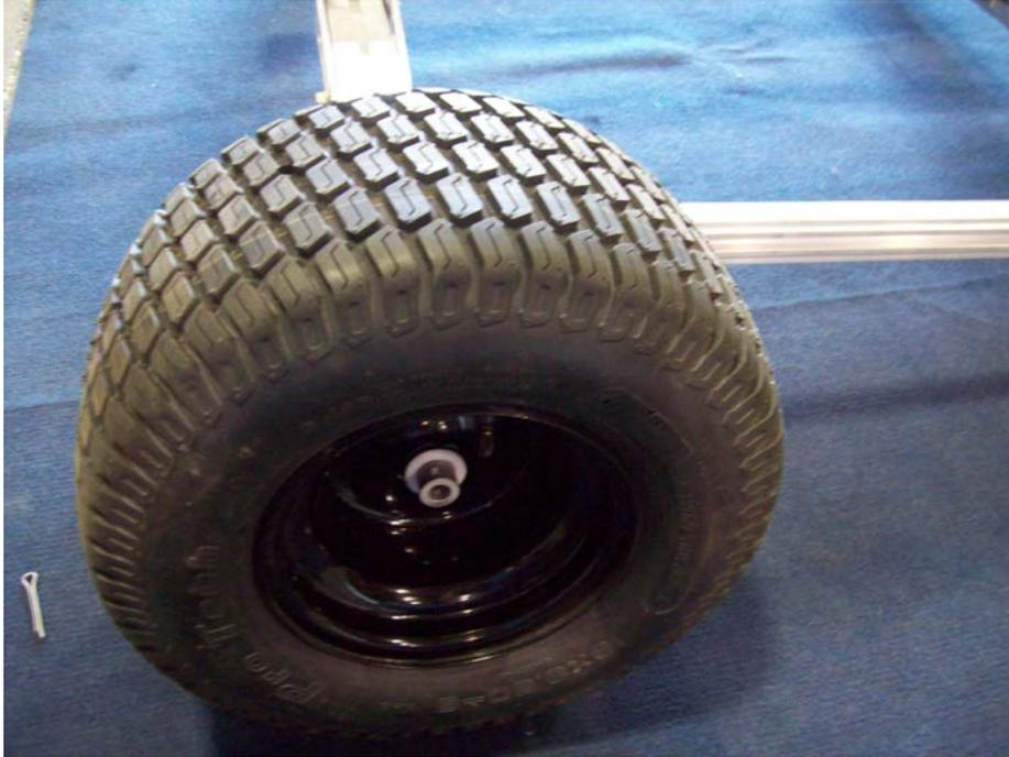
Install the wheels with the valve stems facing out.
