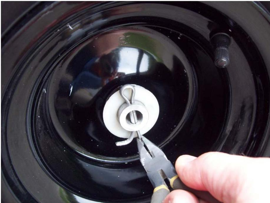
Install the last four nylon washers on each axle with the grooved side facing in. Insert cotter pins and bend the ends so they don't come out.
