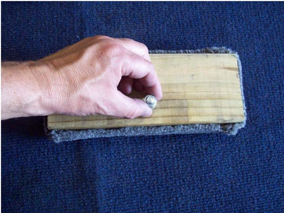
Locate the 10" padded cradle and remove the lock washer and nut from the backside.
