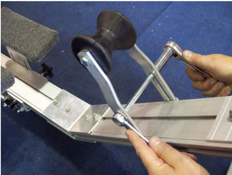
Position bow stop and tighten nuts. Final adjustments will be made when boat is on dolly.
