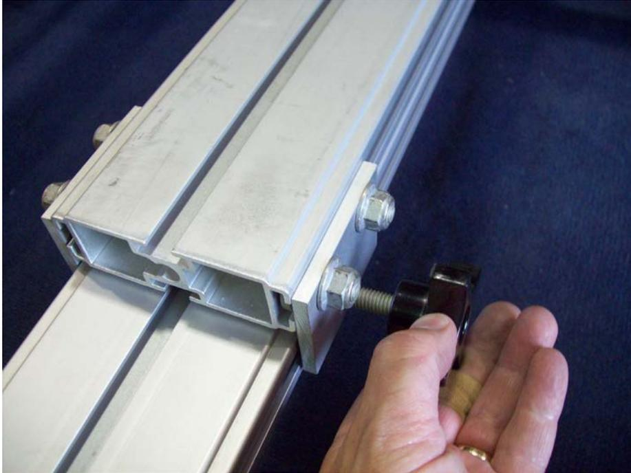
Locate the two, four prong knobs and install them on each side of the rear tongue section.
