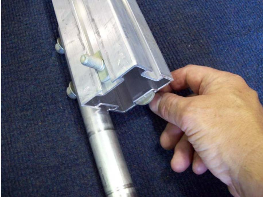
Install two T-bolts on both sides of the axle assembly and repeat for other side.
