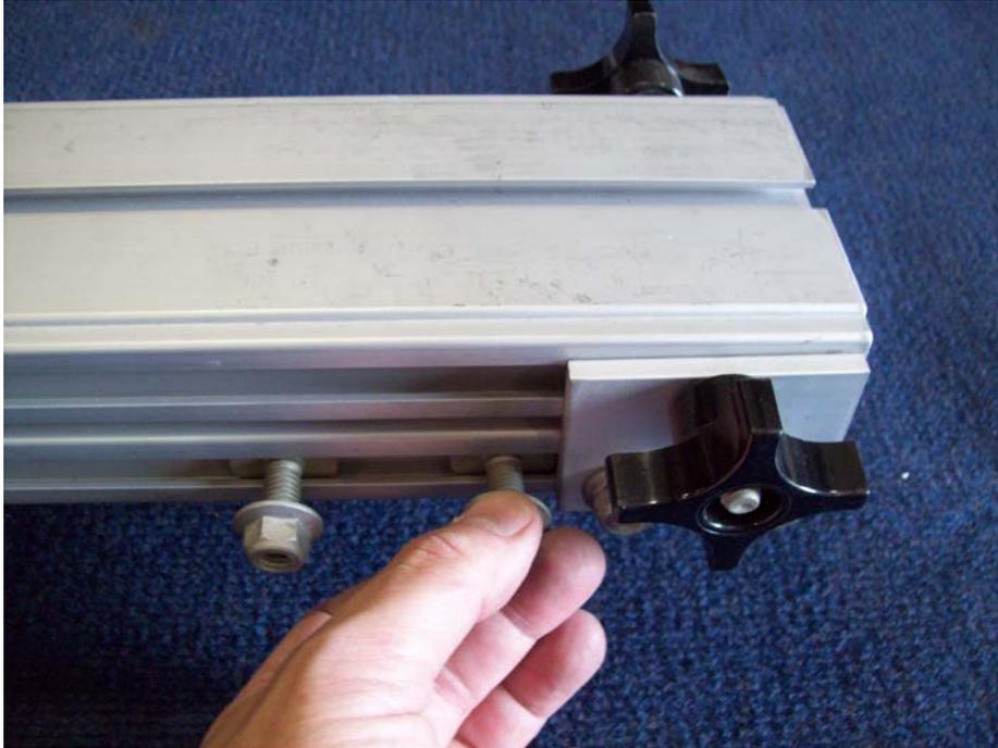
Remove the nuts from both sides of the lower tongue section. Make sure the four prong knobs are on the upper tongue section as shown.
