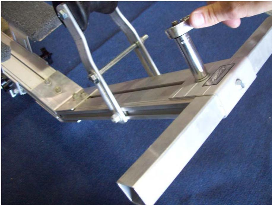
Install handle on the front tongue section and tighten nuts.
