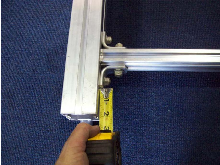
Position the axle spacer 2" away from the end of the axle.
