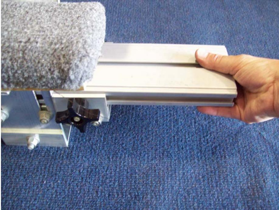
Loosen the knobs on both sides of the tongue section. Slide the tongue section out enough to attach the front tongue section with plates.
