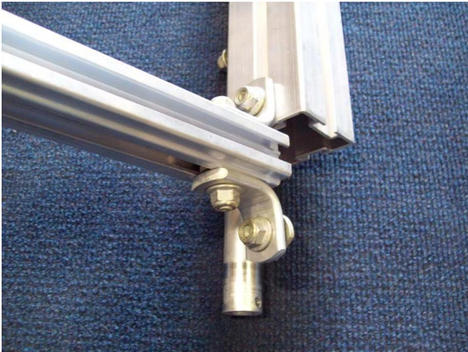
Insert axle spacer into the axle assembly as shown.
