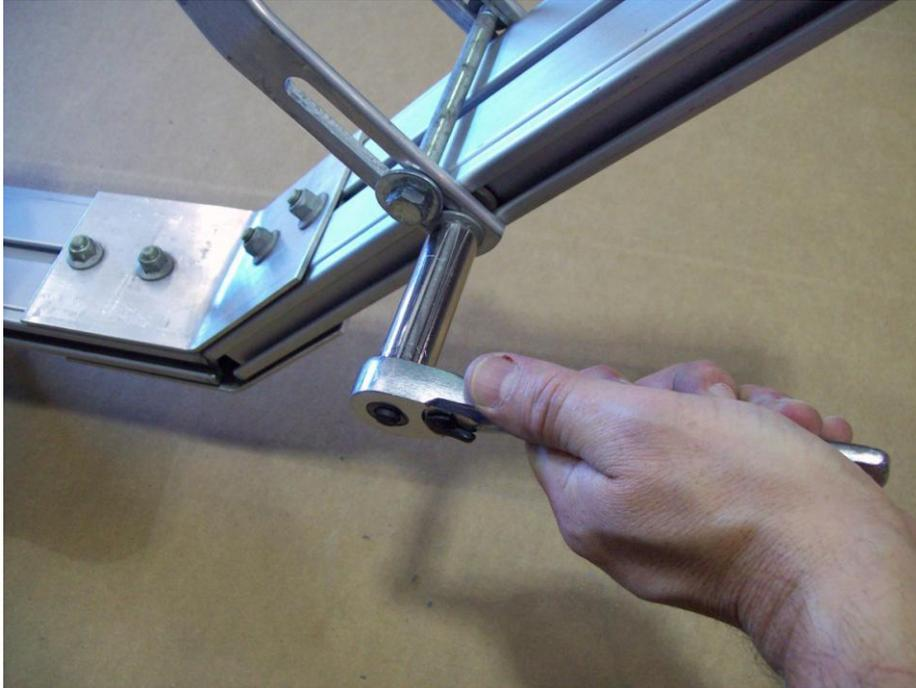
Position bow stop and tighten nuts.
