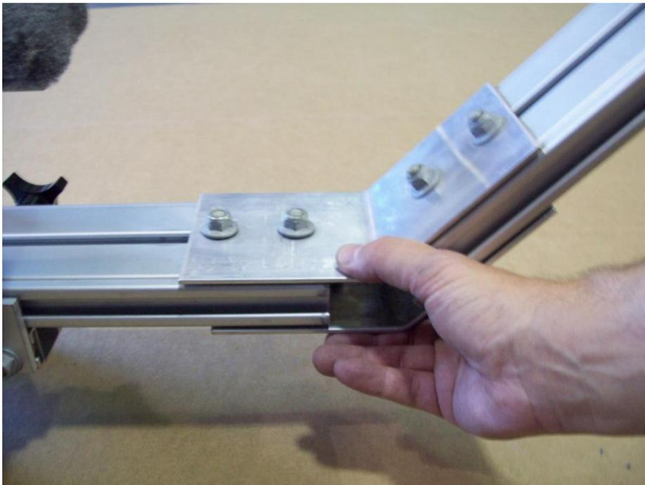
Install front tongue section into upper tongue as shown.
