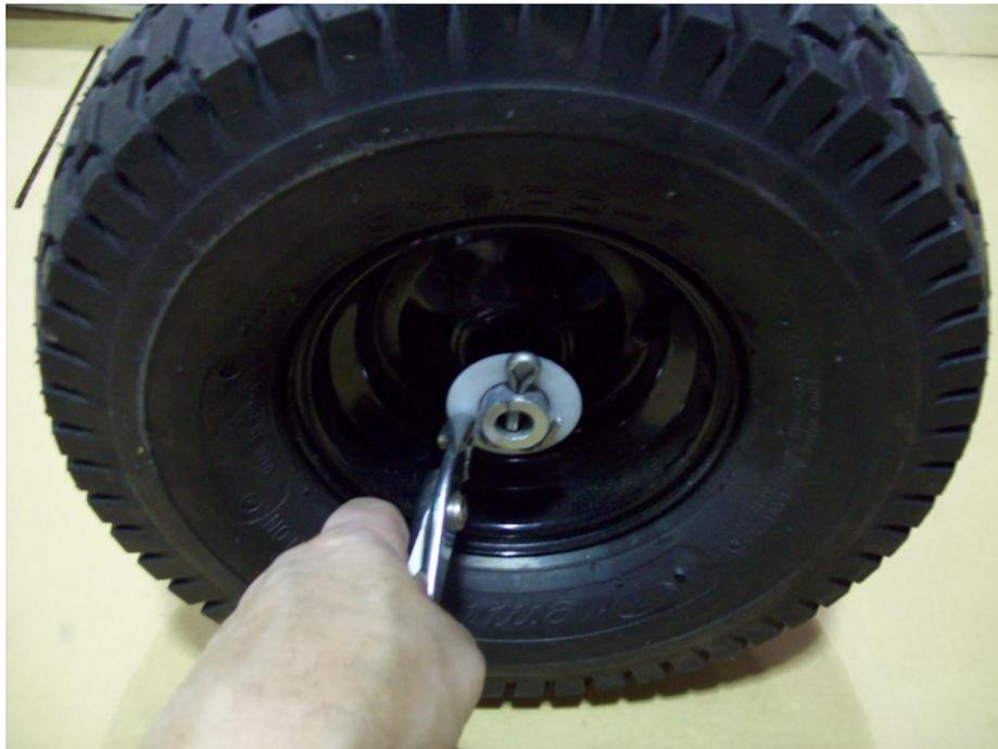
Install the wheel with valve stem facing out. Install the nylon washer on the axle with the grooved side facing in. Insert cotter pin and bend the ends so it doesn't come out. Repeat this process for the other side.
