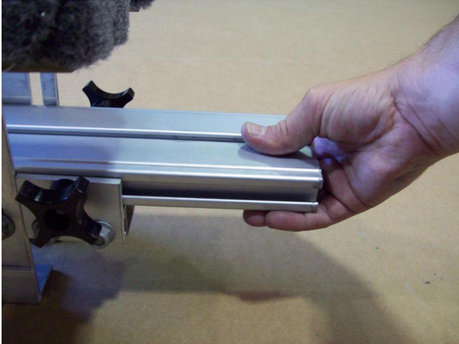
Slide the upper tongue section out enough to attach the front tongue section with plates.
