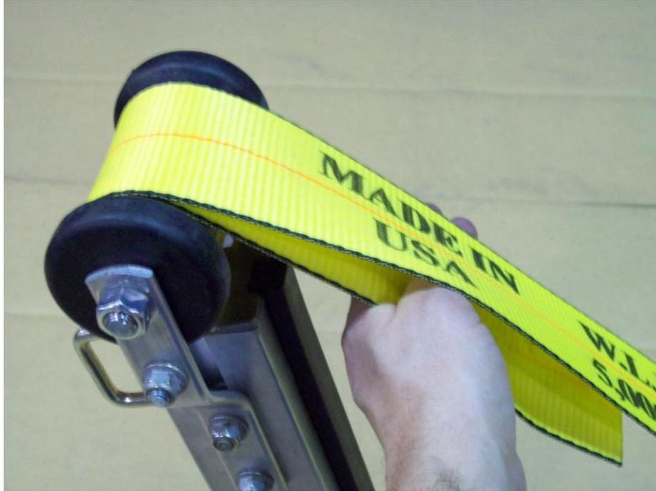
At this point, pull inner strap to raise it up off the axle assembly.
