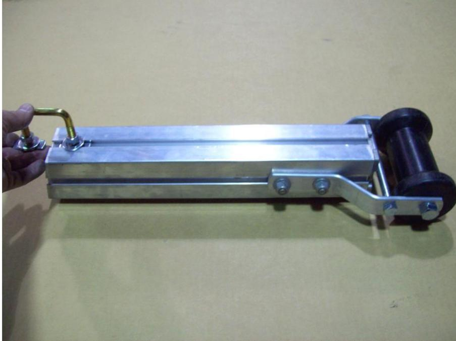
Locate the two upright assemblies. Insert one web strap clip on the back side of the assembly as shown. The clip will face to the outside of the dolly when completed.
