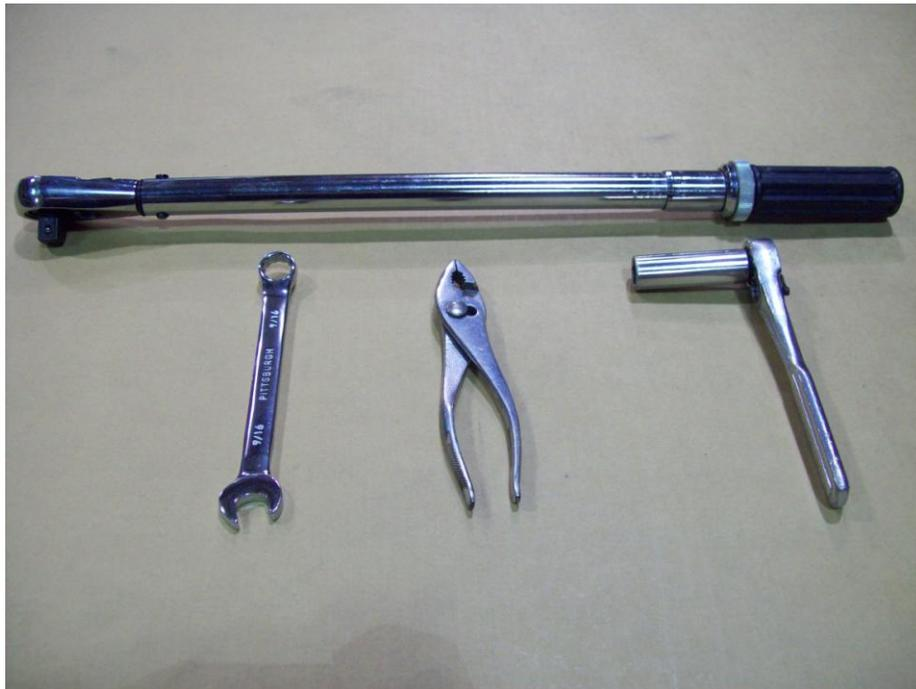
**Open end 9/16” wrench, pliers, ratchet, 9/16” socket, and torque wrench.**
