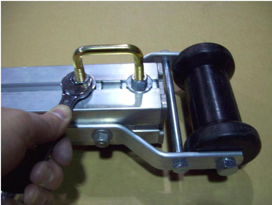
Once web strap clip is in position tighten nuts. Repeat this process for the other side.
