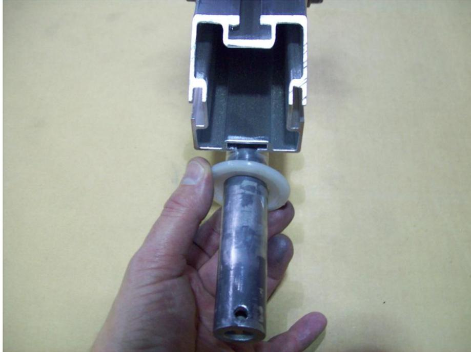
Install one nylon retainer washer on the axle with the grooved side facing out.
