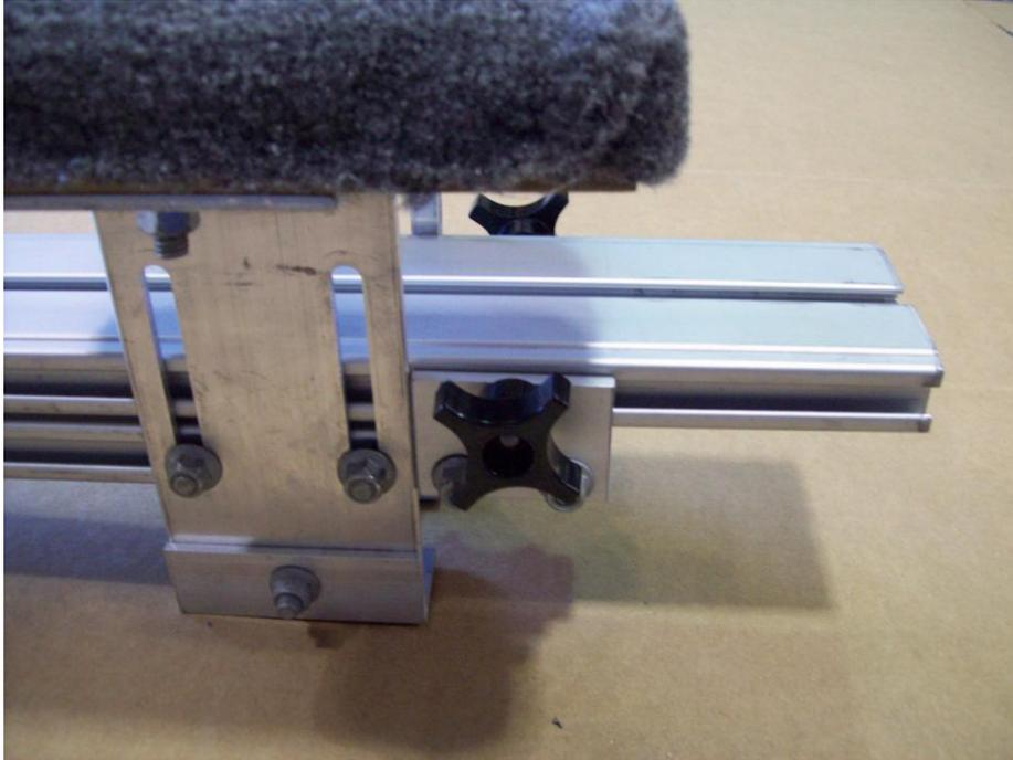
Install 2 four prong knobs on the upper tongue. Leave knobs loose for now until finished.
