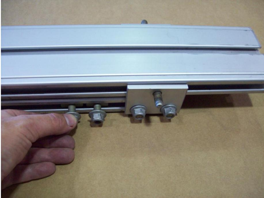
Remove the nuts from both sides of the lower tongue section.
