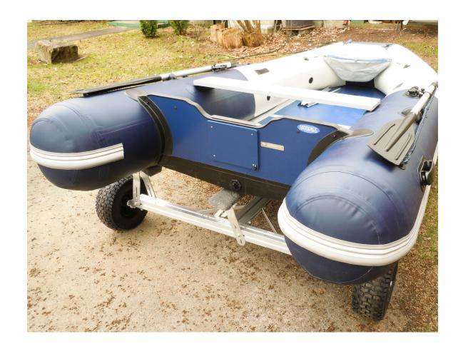
**Adjust Outer Pads to Support the Tubes**
